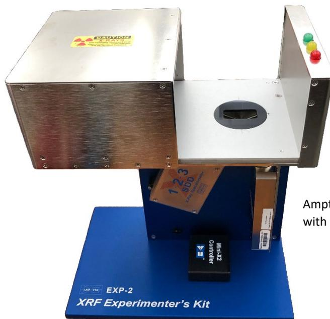
Amptek Experiment's XRF Kit shown with sample enclosure opened.
