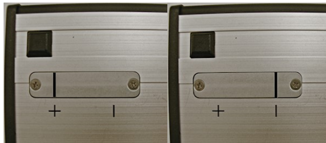
Left: PX5 high voltage jumper set to positive for Si-PIN or CdTe detector. Right: PX5 high voltage jumper set to negative for silicon drift detector (SDD)
