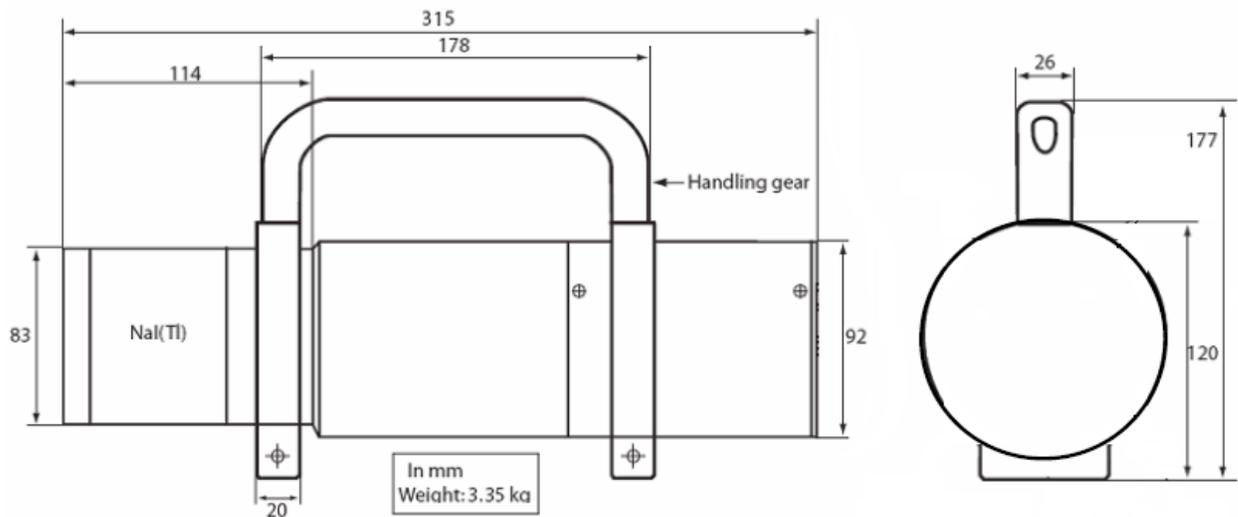
This is for the 76mmx76mm NaI(Tl) scintillator, which is the most common. Contact Amptek for drawings of other configurations.
