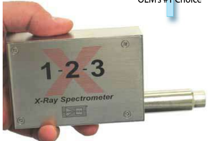
The X-123 is typically used in detecting X-rays with energies from a few keV to 30kV.
