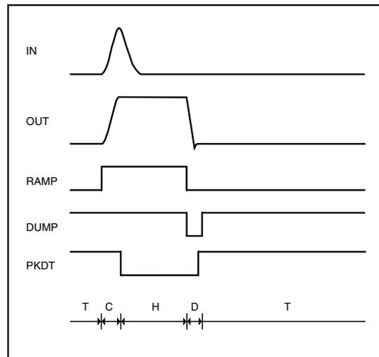
**Figure 4. - Timing diagram illustrating DUMP reset of PH300.**
