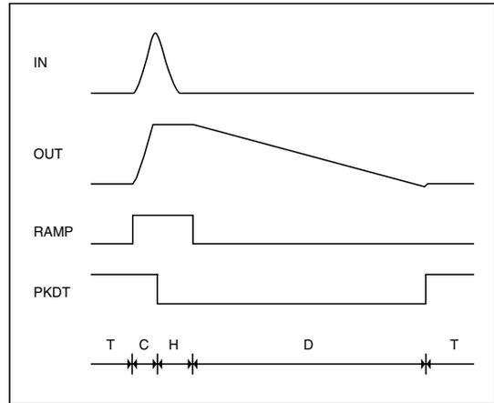
**Figure 3. - Timing diagram illustrating RAMP reset of PH300.**
