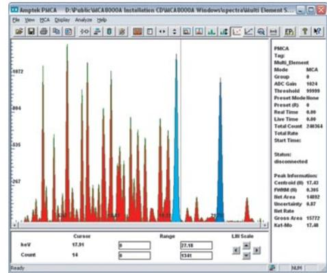
Example of MCA8000A display and acquisition software with interface to XRF-FP quantitative analysis software.
