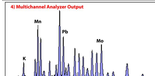
Trace 1 above shows the input to the DP4, which is the output from a reset-type charge sensitive preamplifier. This is processed by the analog prefilter producing the prefilter output shown in Trace 2. This is digitized and then processed digitally, producing the DP4's shaped output shown in Trace 3. Finally, the DP4 creates a multichannel analyzer (MCA) type output spectrum shown in Graph 4.
