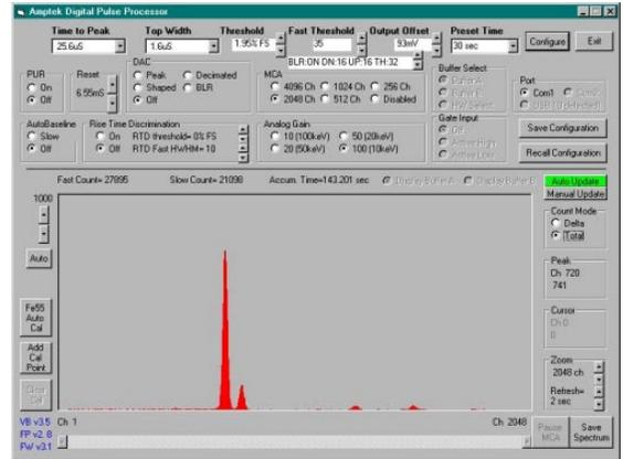
Example of demonstration software supplied with the DP4 for data acquisition (source code provided).
