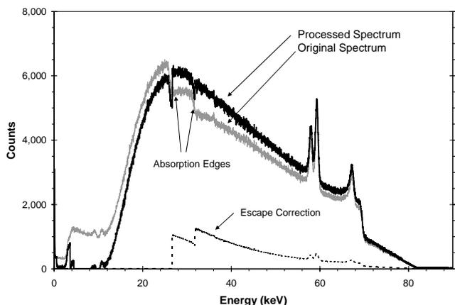
Fig 4. Plot showing the results of the escape peak correction algorithm, applied to a spectrum measured from an 80 kVp tungsten anode X-ray tube. The raw spectrum is shown, with the clear absorption edges and with counts below the expected cut-off due to the filter. Also shown is the escape correction, and then the final processed spectrum.
