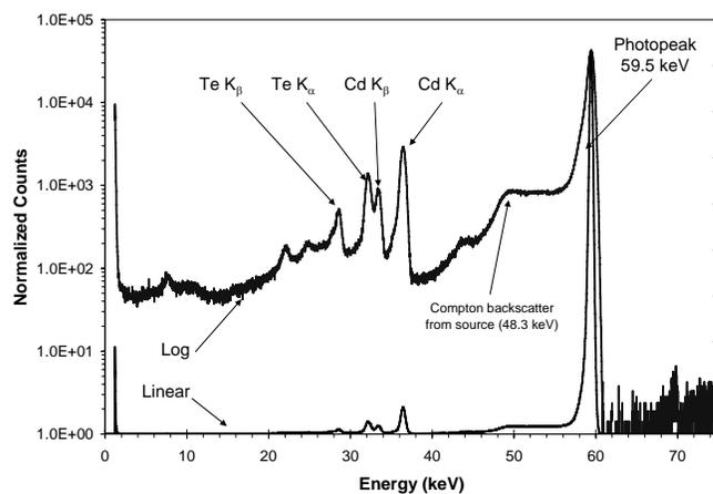
Fig 3. Spectrum measured using a filtered  $^{241}\text{Am}$  source, showing the four escape peaks produced from the 59.5 keV primary peak. Also visible is the asymmetry due to hole tailing and a "shelf" due to photons Compton scattering out of the isotopic source and into the detector.
