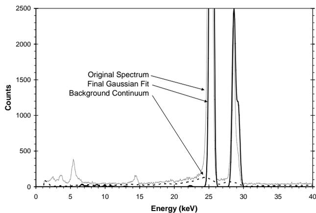
Fig 5. Plot showing Sn characteristic X-rays measured by CdTe. The plot shows the raw spectra, the background continuum which has been removed, and then the Gaussian fits to the resulting spectrum.
