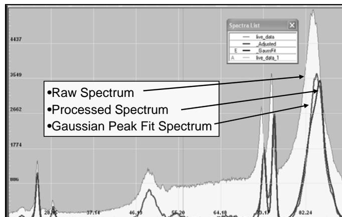
Fig 7. Plot showing the analysis of a Sn-Pb solder, showing the raw spectrum, the processed spectrum after correction for escape peaks and the continuum, and then Gaussian fits to the primary photopeaks.
