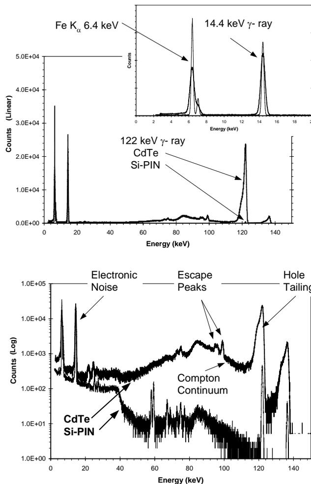
Fig. 1. <sup>57</sup>Co spectrum measured by Si-PIN (thin line) and CdTe (thick line) detectors, both of 25 mm<sup>2</sup> active area. The plot on the top is on a linear scale, with the inset showing the low energy range. The plot on the bottom is on a log scale and illustrates the major spectral features discussed in this paper.
