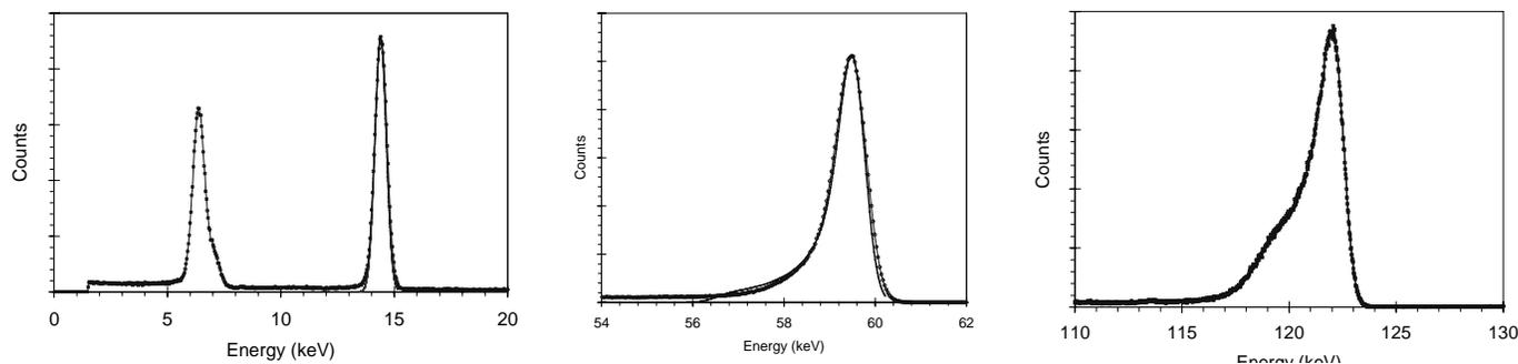
Fig 2. Plots showing the measured and modeled photopeak shape as a function of energy. At 14.4 keV (left), the photopeak is Gaussian. At 59.5 keV (middle), the photopeak exhibits a smooth asymmetric tail to lower amplitudes. At 122 keV (right), additional counts in the tail lead to a step at the anode charge collection efficiency.
