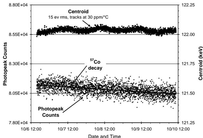
Fig 6. Plot showing stability of the devices at a temperature of 220 K and a bias of 1 kV/mm.
