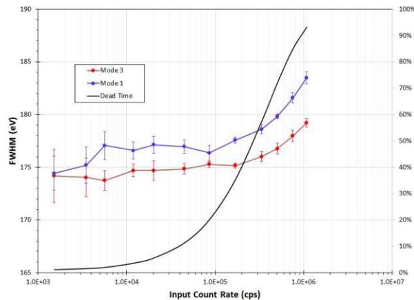
For most users, we recommend retaining Mode 1 as a simple, robust, and good algorithm. For peaking times below  $0.5 \mu\text{s}$ , we recommend Mode 1. For users operating at peaking times above  $0.5 \mu\text{s}$ , at the highest count rates and dead times, and with the tightest stability requirements, we recommend using Mode 3.
