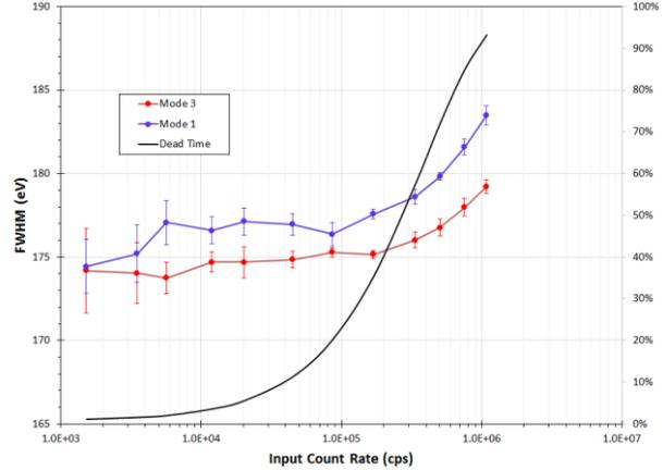
For most users, we recommend retaining Mode 1 as a simple, robust, and good algorithm. For peaking times below 0.5  $\mu$ s, we recommend Mode 1. For users operating at peaking times above 0.5  $\mu$ s, at the highest count rates and dead times, and with the tightest stability requirements, we recommend using Mode 3.
