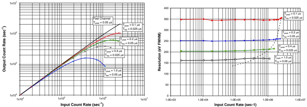
Figure 2. Plot of computed and measured throughput at the highest rates (left) and of resolution versus ICR (right). Data were taken with a collimated Amptek 25 mm<sup>2</sup> SDD and the DP5 with FW 6.02.
