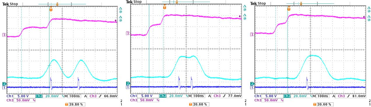
Figure 10. Oscilloscope traces demonstrating fast channel operation. The pink trace is the ADC input. The light blue trace is the fast output (peaking time of 0.1 μsec). The dark blue trace is “ICR”, the logic signal indicating that a pulse was detected in the fast channel.
