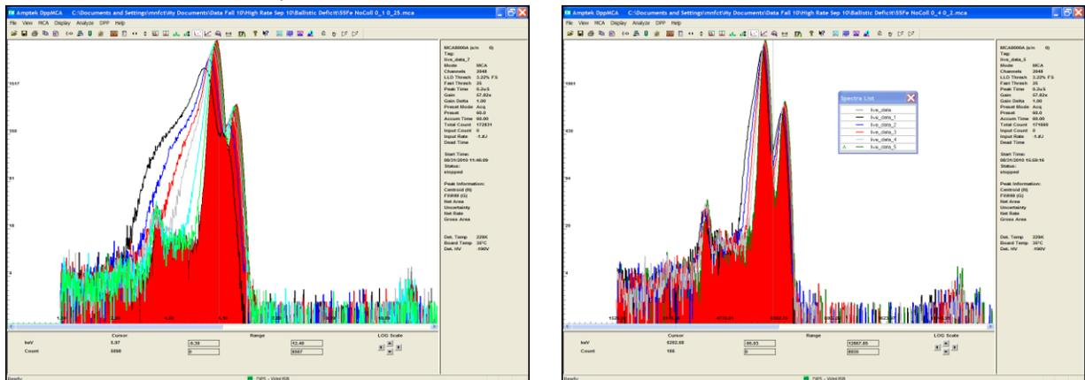
Figure 4. Spectra taken at  $T_{peak}=100$  ns (left) and 400 ns (right) with a DP5 and a 25 mm<sup>2</sup> Amptek SDD.
