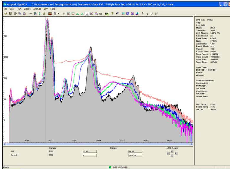
Figure 6. Spectra showing the effects of flat top duration on the shape of the pile-up events. The data were all taken for  $T_{peak}=0.4$   $\mu$ s and at an ICR of 1 Mcps. The orange trace is with PUR disabled. The filled spectrum is with  $T_{flat}=0.2$   $\mu$ s. The other traces are for shorter  $T_{flat}$ .
