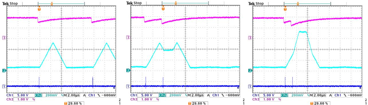
Figure 9. Oscilloscope traces demonstrating pulse pile-up. The pink trace is the ADC input. The light blue trace is the shaped output (here set to a peaking time of 2.4  $\mu$ sec). The dark blue trace is “ICR”, the logic signal indicating that a pulse was detected in the fast channel.
