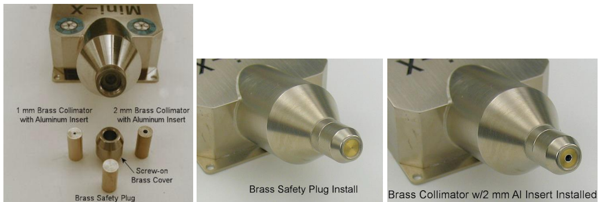
Figure 9. Left photo shows the Mini-X2 collimators, safety plug, and cover. The middle photo shows the safety plug installed in the cover and attached to the Mini-X2. This configuration meets the radiation requirements discussed above. The Mini-X2 ships from the factory in this configuration. The right photo shows the collimator installed in the cover.
