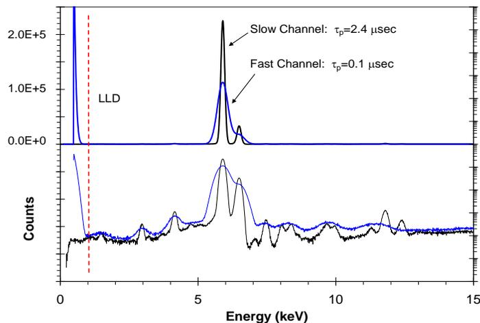
Figure 5 Plot showing spectra measured for the slow channel, at 2.4  $\mu$ sec and 0.1  $\mu$ sec  $T_P$  for the slow and fast channels, respectively. The same data are depicted in linear (top) and log (bottom) scales. Also shown is the LLD for the fast channel.
