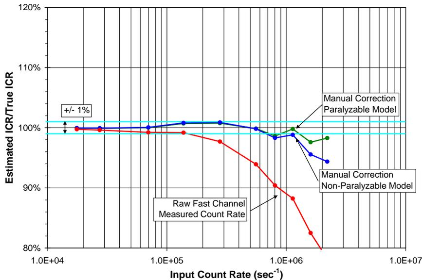
Figure 4. Plot comparing the SDD/DP5 deadtime correction methods.
