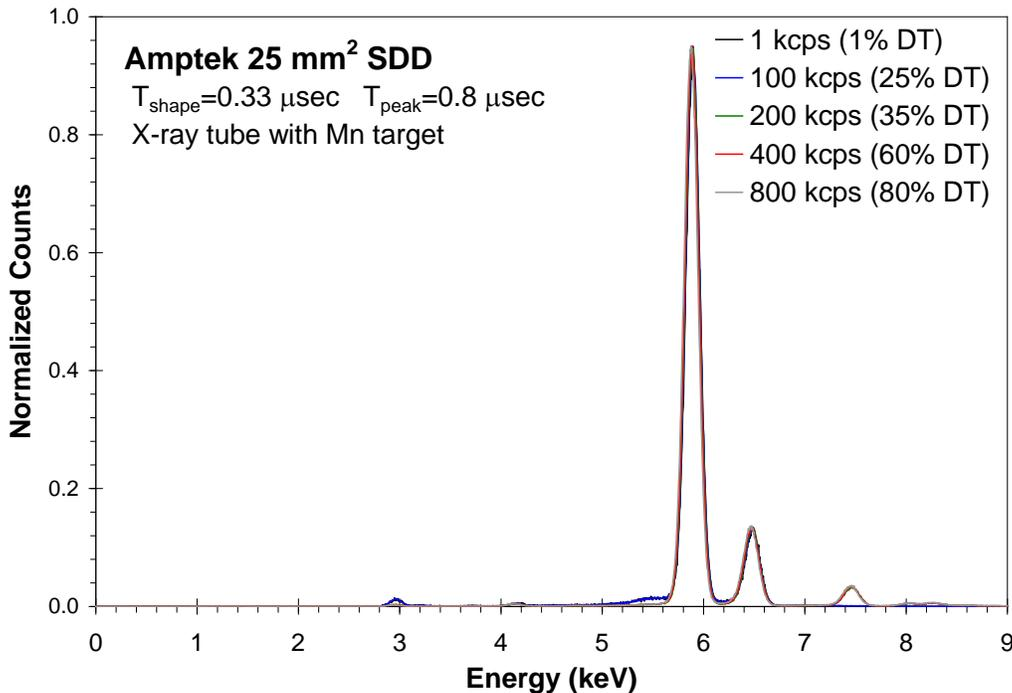
Figure 3. Spectra from a pure Mn target, taken using an SDD with DP5 at  $T_{peak}=0.8 \mu\text{sec}$  peaking time. The data were taken at  $R_{in}$  of 1 kcps (99% throughput), 400 kcps (40% throughput, near the peak of the  $R_{out}$  curve), and 800 kcps (20% throughput, past the peak of the  $R_{out}$  curve). The resolution was 160 eV FWHM.
