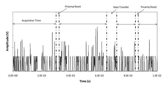
Figure illustrating acquisition time and real time. In this interval, the real time is 10 milliseconds. No counts are measured during the two preamp resets or during the data transfer interval, so the acquisition clock is gated off during these times. The acquisition time in this example is 9.89 milliseconds.
