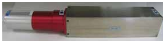
The photo above shows a high sensitivity detector, a 10 \times 10 \times 40 \text{ cm}^3 ( 4 \times 4 \times 16 inch) NaI(Tl) "bar."
