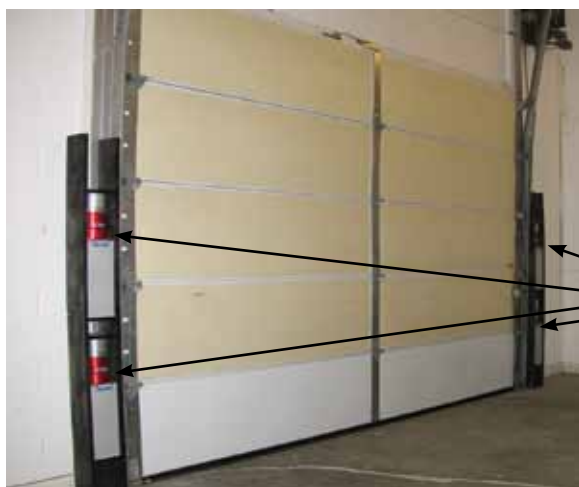
The photo above shows a high sensitivity detector, a 10 \times 10 \times 40 \text{ cm}^3 ( 4 \times 4 \times 16 inch) NaI(Tl) "bar."
