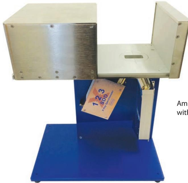
Amptek Experiment's XRF Kit shown with the sample enclosure opened.
