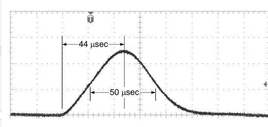
An oscilloscope trace of a PX4 shaped pulse is shown below (20  $\mu\text{sec}/\text{div}$ ). The risetime is well defined at 51  $\mu\text{sec}$ . The pulse is triangular, so is symmetric and has duration 51  $\mu\text{sec}$  (FWHM). The noise bandwidth is comparable to that of a quasi-triangular shaper with the same risetime, so 23  $\mu\text{sec}$ . It will have pile-up properties similar to those of the PX2 output above, but slightly larger noise bandwidth and therefore lower noise.
