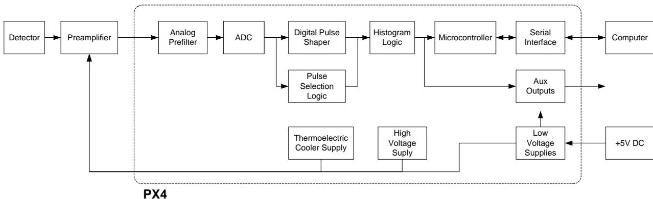
Figure 2. Block diagram of the PX4. It includes the same functions as a traditional system, but in a single, compact module. Digital processing permits greater flexibility in the configurations and makes changing configurations easier.
