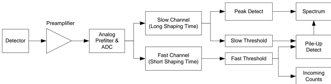
For most detectors, electronic noise is minimized at a fairly long shaping time constant. For Amptek’s XR100 Si detectors, minimum noise is found with a peaking time of 20 to 50  $\mu\text{sec}$ . So the slow channel is
