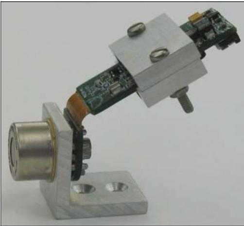
Figure 9. PA230 flexible preamplifier with detector, heat-sink, and mounting hardware.
