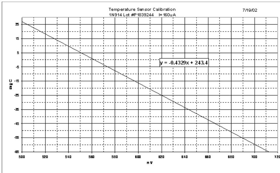
Figure 3. Temperature diode calibration curve for I = 160  $\mu$ A.
