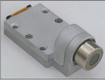
Figure 13. PA-230 Housing. The PA-230 can be ordered with a housing that completely shields the detector and preamplifier and provides heat-sinking and mounting holes. This optional housing saves the OEM the design time of fabricating a custom enclosure.
