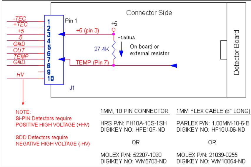
Figure 2. PA-210/PA-230 Connection Diagram.
