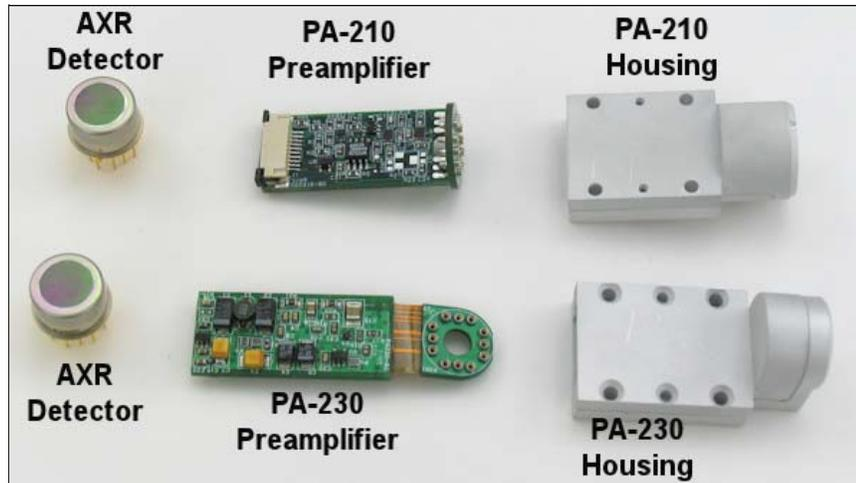
Figure 1. AXR Detector, PA-210 or PA-230, Housing.
