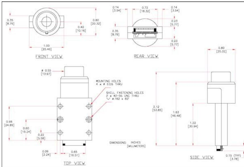
Figure 8. AXR/PA-210 with housing mechanical dimensions.
