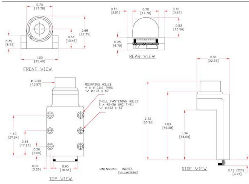
Figure 14. AXR/PA-230 with housing mechanical dimensions.
