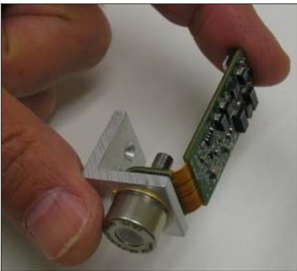
Figure 10. PA230 flexible preamplifier with detector and heat-sink.
