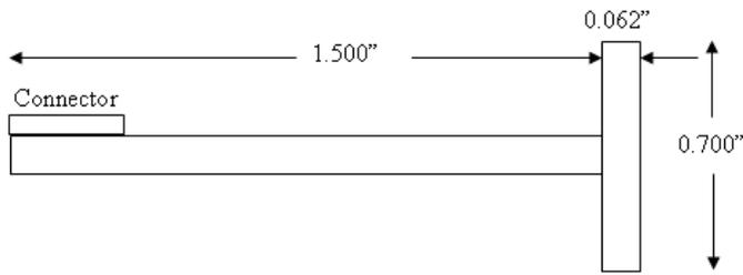
Figure 6. PA210 preamplifier mechanical dimensions.
