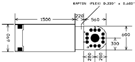
Figure 12. PA230 Mechanical dimensions.
