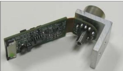
Figure 11. PA230 flexible preamplifier with detector and heat-sink.
