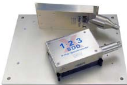
The Mini-X mounted on MP1 with X-123SDD.
