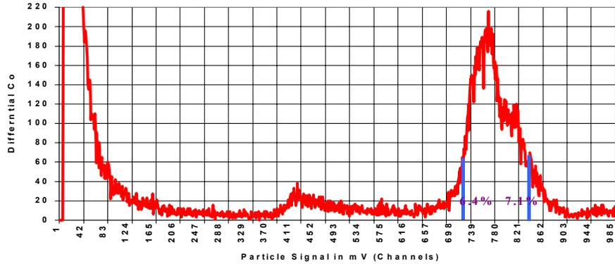
Fig. 3 Resolution of Instrument C  $R_L = 6.4\%$   $R_R = 7.1\%$
