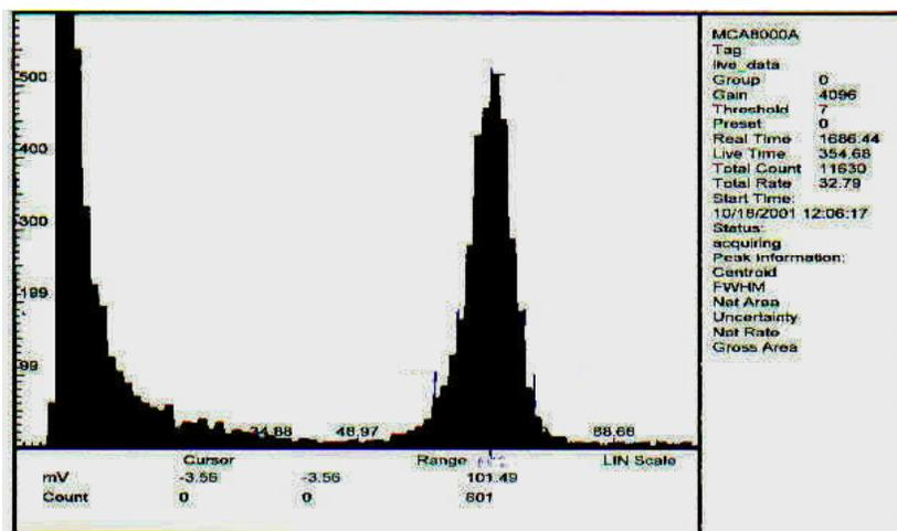
Fig. 2 Resolution of Instrument E  $R_L = 11.3\%$   $R_R = 10.2\%$
