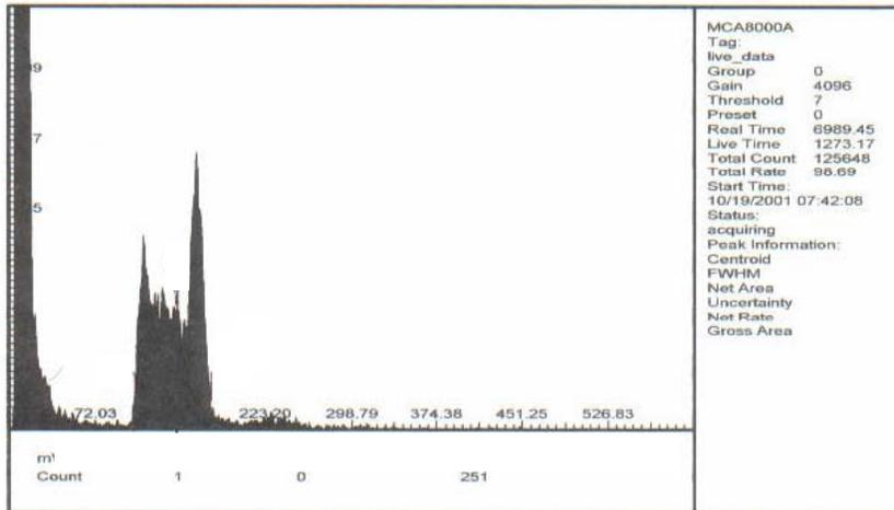
Fig. 1 Resolution of Instrument A  $R_L = 22\%$   $R_R = 22\%$
