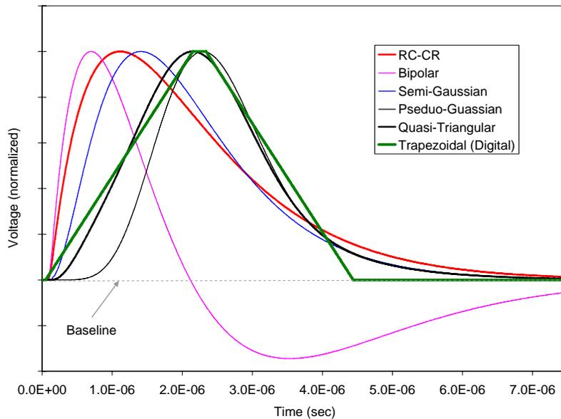
Figure 2. Illustration of pulse shapes obtained with different shaping amplifiers. Each of these has a “shaping time constant” of 1  $\mu$ sec but the the integrators, the low pass filters, use different transfer functions. The general properties are as follows:
